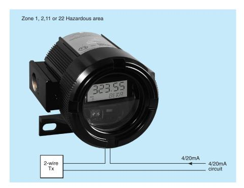
The BR323AL and BR323SS are flameproof field mounting loop powered indicators that only introduces a 2.3V drop making them suitable for inclusion in almost any 4/20mA loop. The two instruments are electrically identical but have different enclosure materials. The BR323AL is housed in an epoxy painted aluminium enclosure and the BR323SS in a 316 stainless steel enclosure. Both provide IP66 and NEMA Type 4X protection.
